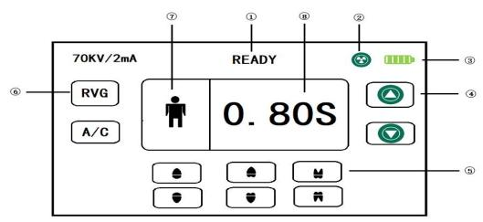
1 Standby display: Indicates that it is in standby state and can be exposed normally.
