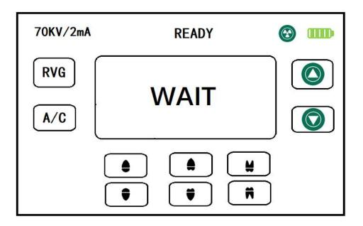
6. After exposure, the standby protection status, to 20 s, 20 s after restores last exposure Settings; Before that, in addition to the power switch, all keys are in the locked state.
