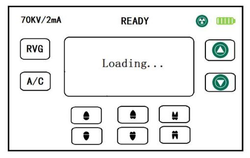
2. In the process of loading equipment will start self-checking function, If have the failure will display failure code (please see note 4.5 fault code specific fault code), are shown in figure 1 below: If trouble-free, into the normal state, as shown in figure 2:
