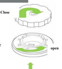
do not overflow; clockwise rotate the softener cover to prevent salt leakage from corroding the inner tank. If salt is spilled on the bladder, the procedure must be run to flush once,
