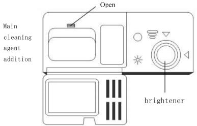
When the brightener is filled about 100 ml, the number 1-6 at the place where the brightener is used can be added several times at one time. The factory default value is position 4. If the light effect is not ideal, the rotary knob can be used to adjust the amount of standard brightener 4 ml.
