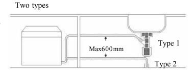
drainage pipe should be not higher than  $600\,\mathrm{mm}$  , not lower than  $300\,\mathrm{mm}$ .
