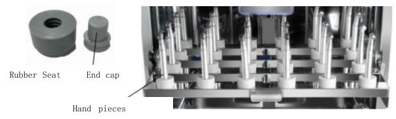
The hand pieces are inserted directly into the rubber seat of the rack. Please do not put it to the bottom to prevent water from flowing into the hand pieces. The rack can clean at most 24 hand pieces each time. when the machine working, you could cover the end cap on the rubber seat.
