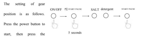
start/ pause button within 60 seconds for more than 5 seconds to enter tap position setting mode, if not press start/ pause button within 5 seconds, which will quit the setting mode.
