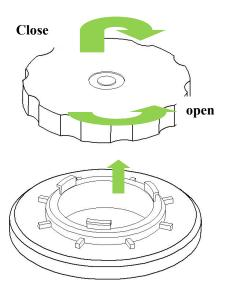
the water softener, do not overflow; clockwise rotate the softener cover to prevent salt leakage from corroding the inner tank. If salt is spilled on the bladder, the procedure must be run to flush once.
