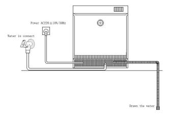
3. Turn on the tape. Open the water valve (keep the water be on during washing).
