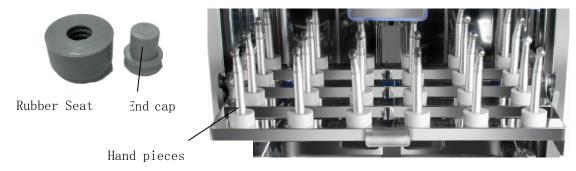
The hand pieces are inserted directly into the rubber seat of the rack. Please do not put it to the bottom to prevent water from flowing into the hand pieces. The rack can clean at most 32 hand pieces each time. when the machine working, you could cover the end cap on the rubber seat.
