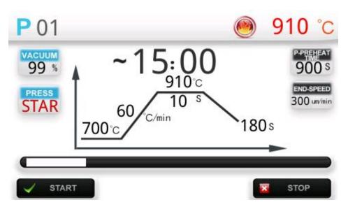
When the system is in **standby mode**, press "**PRESS INGOT**" button to enter the die casting interface. At this time, the necessary items such as embedding ring, casting block and push rod should be ready. After placing the embedding ring, press [start] to start a die casting process. The "press" position shows the die casting status, "N / C" is the preheating status, "star" is the start of die casting, and "end" is the completion of die casting.
