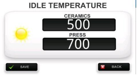
**Idle temperature** is Porcelain furnace PRESS not in firing ,a temperature value user hope to it static.
