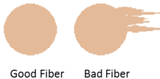
Figure 3.11 Aiming beam spot emitted from good fiber compares with that from bad fiber
