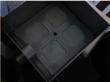
Clean the non-woven fabric filter which is under the board
